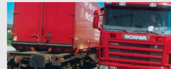
The container is placed on the railway wagon and the Mobiler elements are pushed back onto the truck.
