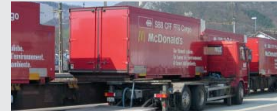
The truck with the mounted Mobiler parks alongside the railway wagon.
